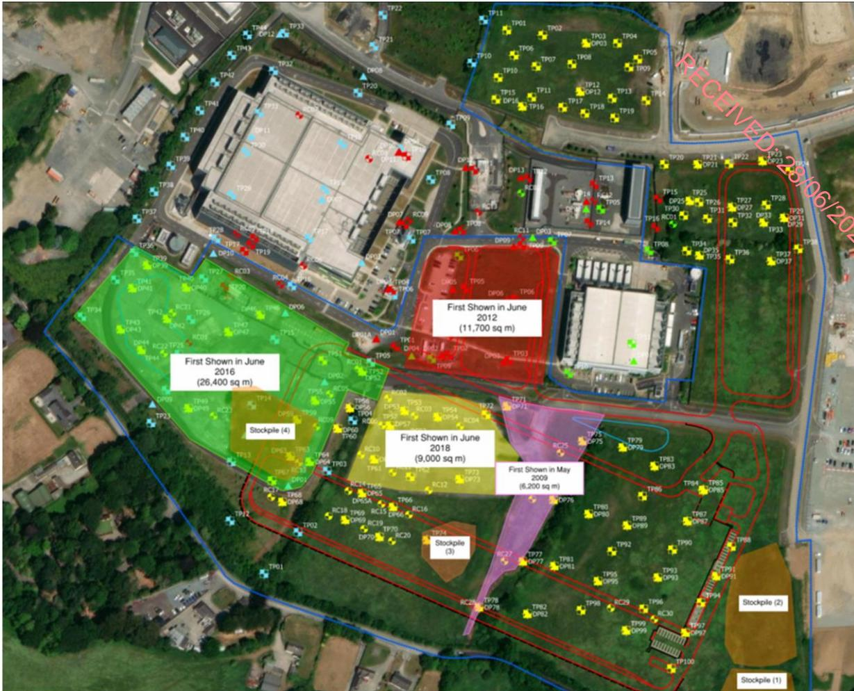
**Figure 2: Areas of made ground materials based on aerial photography and completed ground investigations, identified stockpiles.**
